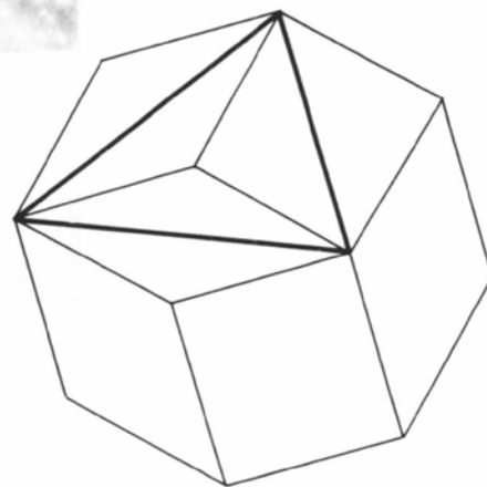
Fig. 7. (111) section through the rhombic dodecahedron. Notice the triangular-shaped intersection (shown by thick lines) representing the observed diffuse intensity distribution in this orientation.
